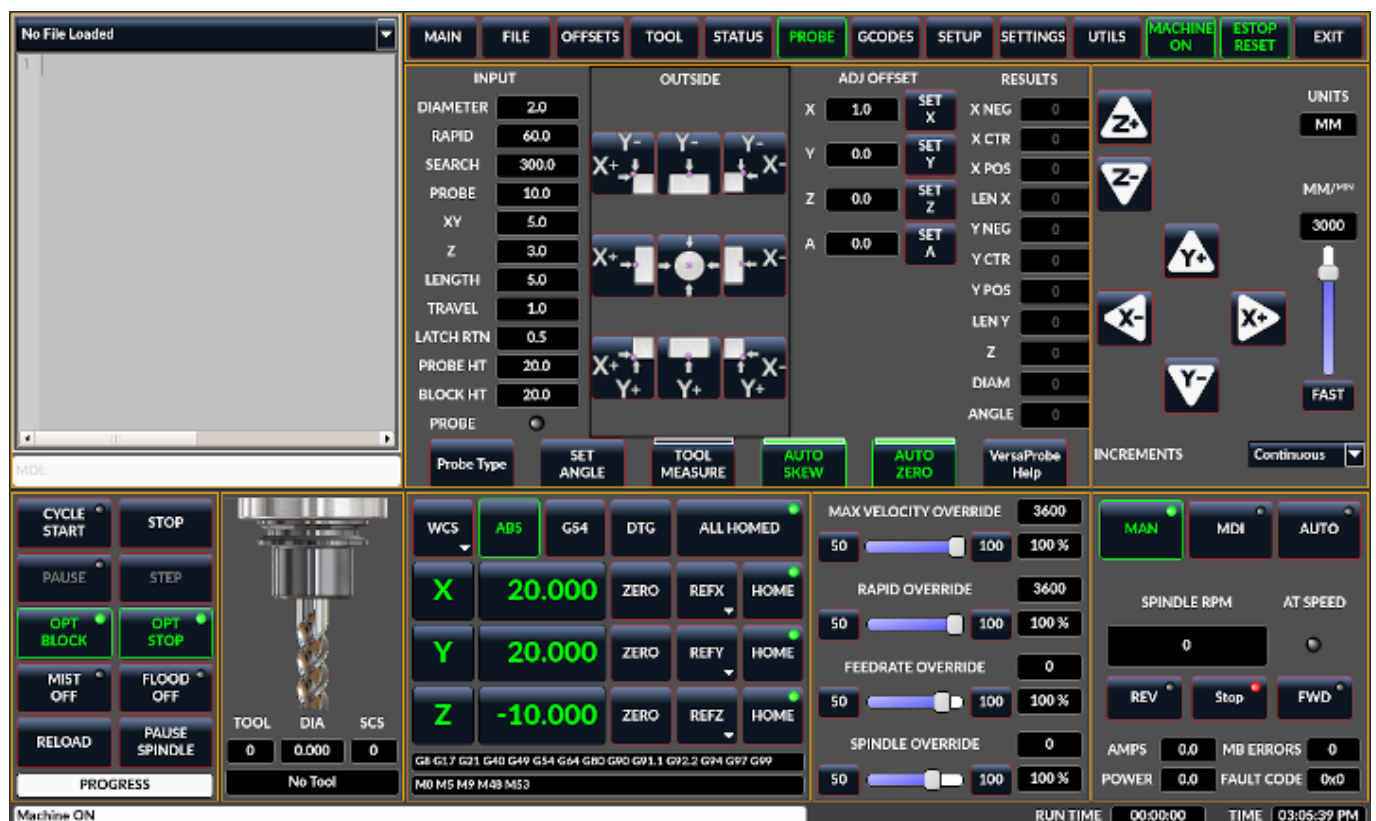
Figure 10.29 - QtDragon - Versa Probe Option
