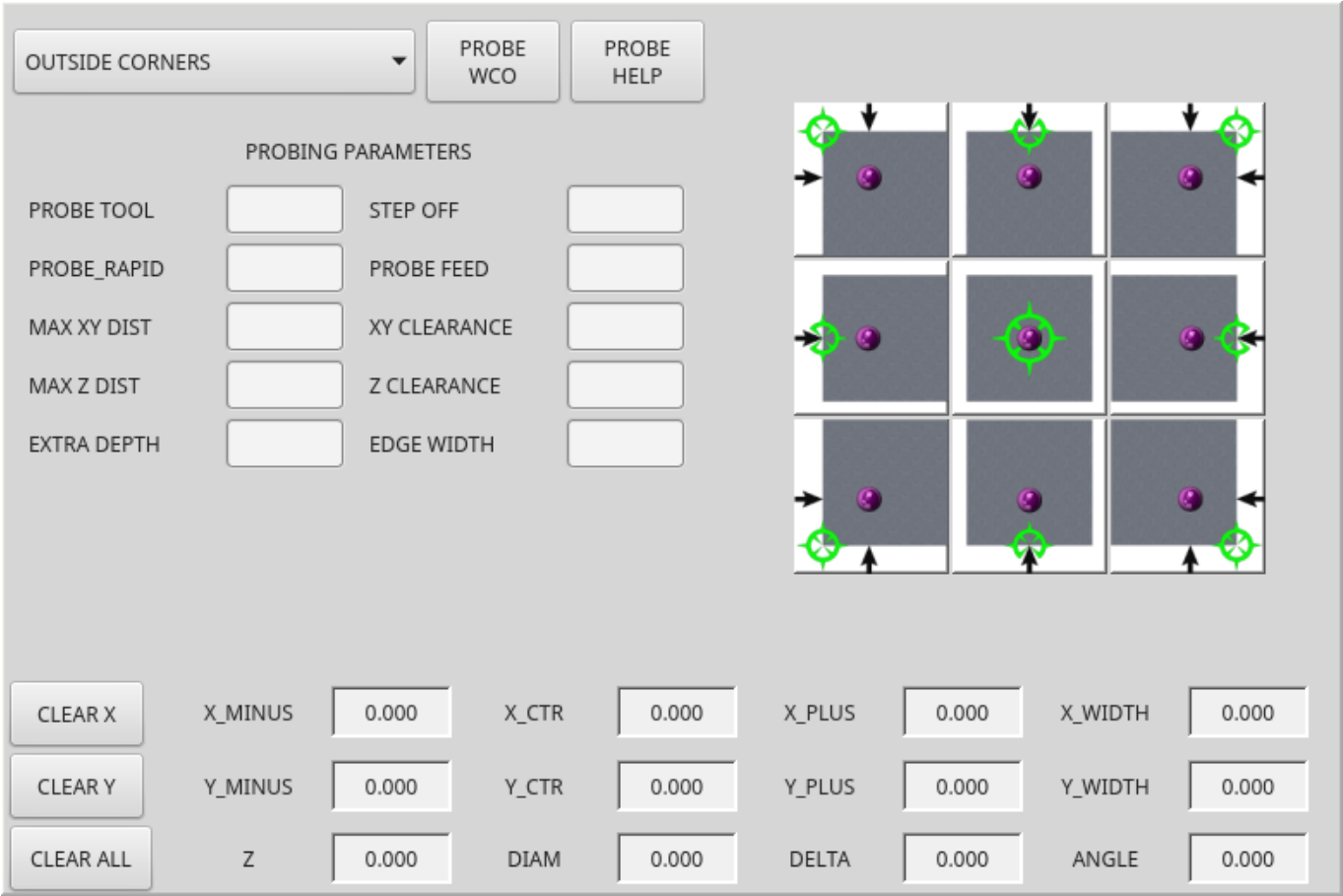
Figure 12.93 – QtVCP BasicProbe: Simple Mill Probing Widget
