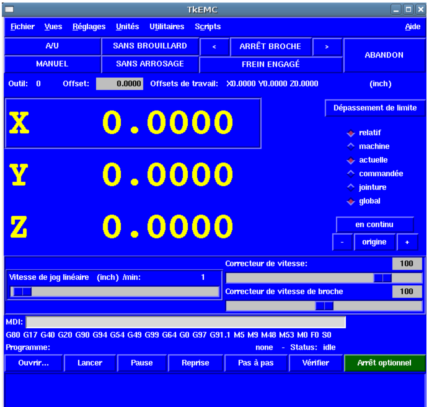
Figure 2.7 - TkLinuxCNC graphical interface
